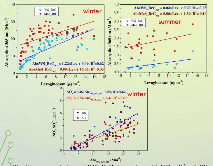
Significant correlations of WS\_BrC absorption with  $NO_3^-$  ( $R^2 = 0.62$ ) and  $SO_4^{2-}$  ( $R^2 = 0.57$ ) in winter imply secondary formation of water-soluble light-absorbing compounds.
