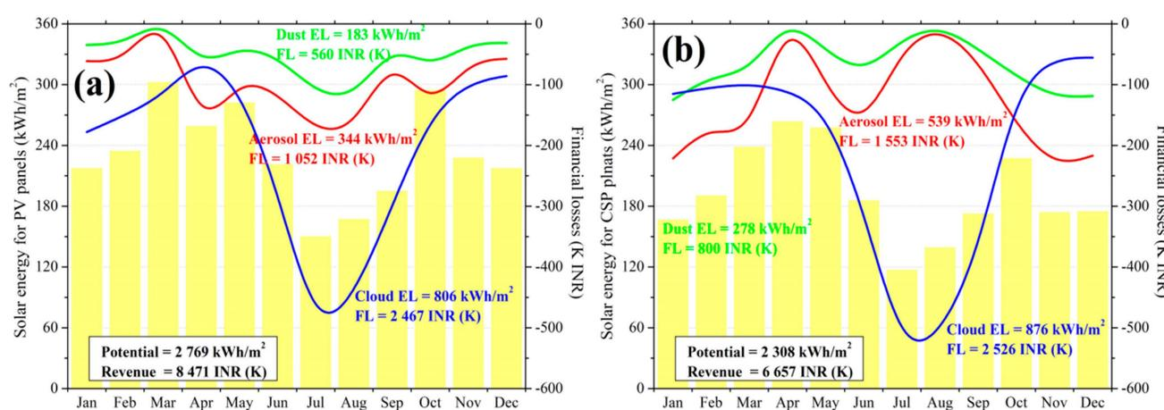
**Figure D:** Financial analysis of the aerosol, dust, and cloud impacts on the produced solar energy from PV (a) and CSP (b) installations with nominal power of 1 MW in the region of Nainital. The impact was quantified in terms of monthly mean and total energy losses, financial losses, and solar energy potential.
