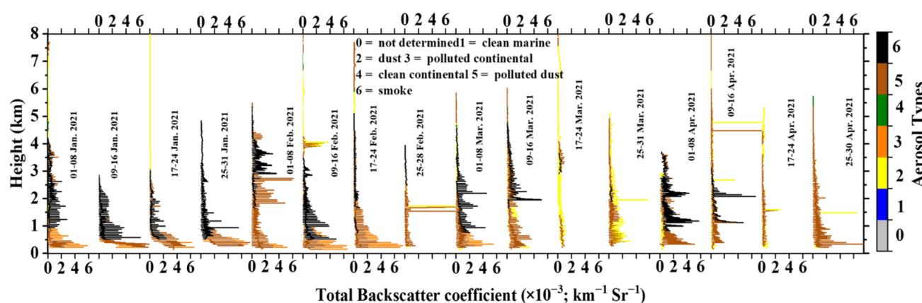
**Figure A:** Weekly mean vertical profiles of the total backscattering coefficient during January to April 2021. The color bars show the aerosol type.
