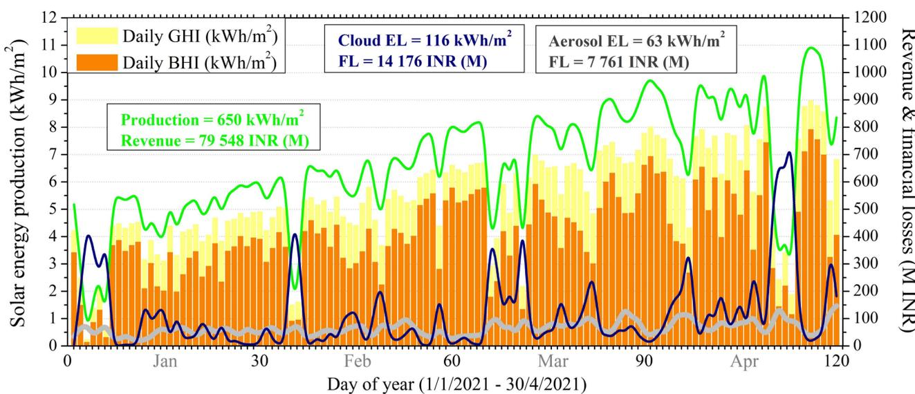
**Figure C:** Financial analysis of the aerosol & cloud impacts on the produced solar energy during Jan to Apr 2021. The impact was quantified in terms of daily mean and total energy losses, financial losses and solar energy potential.
