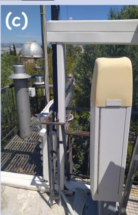
Figure 1: Photo of the measuring site (a) in Athens city center, (b) aethalometer (AE-33) and (c) CL-31 ceilometer.
